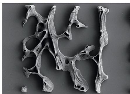
Fig. 2: SEM imaging of an Osteoprint prepared by slice-by-slice 2PP of the hybrid ceramic Ormocomp<sup>®</sup> photoresist.
