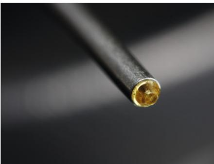
Figure (b): This nozzle is mounted into a metallic syringe tip.
